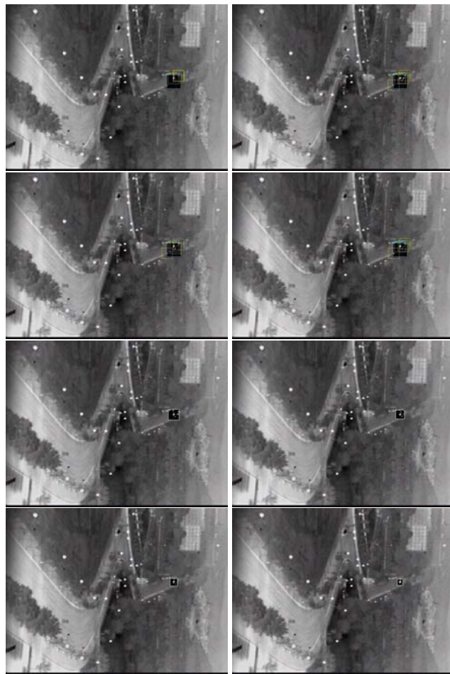
Figure 5: Green rectangle shows the initial search area. Yellow rectangles are candidate targets. White rectangle is selected one that have the highest probability after couple of frame sequences. 8 frame sequence is presented from initial frame.
